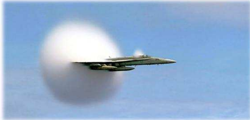
Figure 1.5: Snapshot of shock condensation effect around the jet fighter Boeing F-18 (Hornet) at transonic flight in humid air. It arises during acceleration when the air flow at some parts of the fuselage reaches supersonic speeds. When the resulting shock wave detaches, it builds up a sudden rarefaction that, lowering the temperature, causes condensation of the ambient water vapor.[Courtesy: J. GAY, U.S. Navy] A similar picture was recently taken from an F-4 (Phantom II) during an air show at Point Magu Naval Air Station, CA. (The MilitaryAircraft Archive, http://www.milair.simplenet.com/ )
